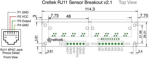
All dimensions in millimeters. Tolerance ±0.5 mm.Specifications subject to change without notice.© 2015-2017 Creltek
